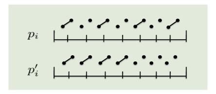
freq(p) is the frequency vector (of length |E|) representing the number of times each edge occurs in the interval p of the partition.
