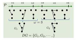
A dynamic Graph is a time series of Graph snapshots. Each snapshot represents a state of the system over an interval of time such as a minute, a day, or a year in the life of the system.
