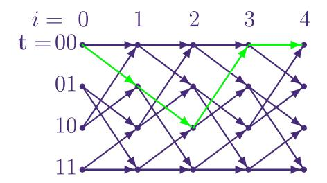
Green path corresponds to the system  $\{0, 0, 1, 0\}$  and the weight of the path is the performance measure of this system.
