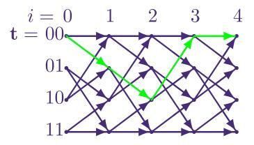
Green path corresponds to the system  $\{0, 0, 1, 0\}$  and the weight of the path is the performance measure of the system.
