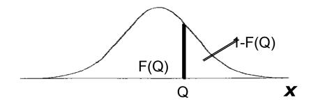
C<sub>o</sub>=c-v: overstocking cost  $C_u$ =p-c: understocking cost F(Q): service level  $C_o * F(Q) = C_u * [1- F(Q)]$   $F(Q^*) = \frac{C_u}{C_u + C_o}$
