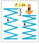
Since, from Newton's second law of motion, we also know that F = ma (mass  $\times$  acceleration), and a(t) = x''(t), we get the following basic mathematical model for a spring-mass system<sup>2</sup>:
