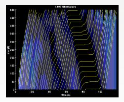
Shock wave on I-680 in Walnut Creek, CA, during rush hour [Coifman]. The graph shows distance traveled (vertical axis) as a function of time (horizontal axis).
